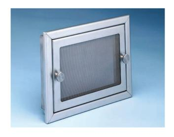
The robust stainless steel frames of the particulate filter are worked from one piece and backed with a tight wire mesh pursuant to DIN ISO 4783. Mesh size 0.5 x 0.32 mm. The mounting frame is secured by solid stainless steel knurled screws (20 mm border, plus 10 mm support). SL particular filters meet the requirements of DIN 1946, Part 4.
